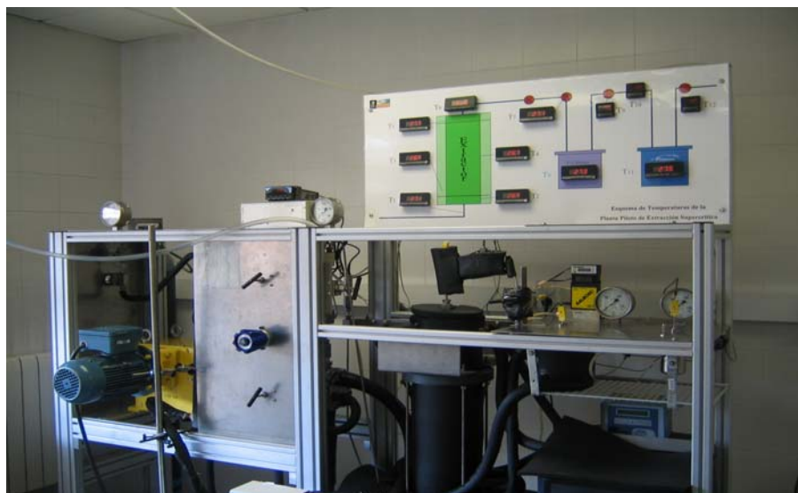
Figure 1. Pilot plant of supercritical extraction GATHERS, Universidad de Zaragoza.
